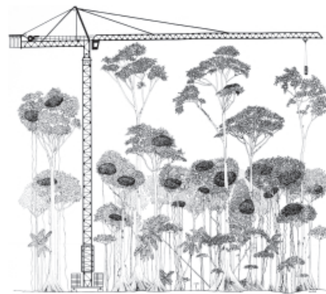
Fig. 14. Diagram showing a canopy crane in a tropical rainforest (archives of the Smithsonian Tropical Research Institute).
