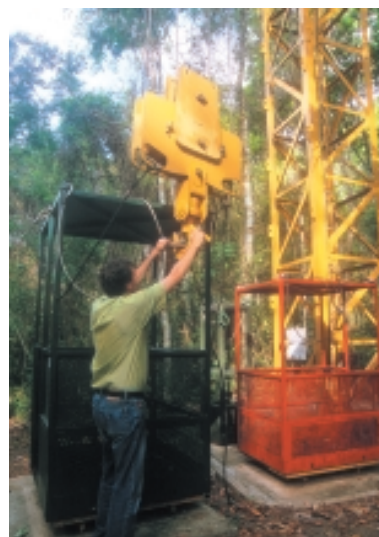
Fig. 16. Connecting the crane hook to the gondola at Parque Natural Metropolitano in Panama (photo Marcos Guerra).
