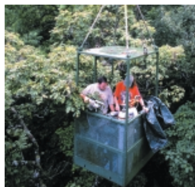
Fig. 17. Measuring leaf uptake of reactive nitrogen, Jed and Kimberlee Sparks, researchers from Cornell University, make leaf-level measurements of photosynthesis and reactive nitrogen uptake from the San Lorenzo crane in Panama (see Chapter 4.3.5). From the gondola, large amounts of equipment including compressed gas cylinders, a photosynthesis system and a device for measuring trace amounts of gaseous reactive nitrogen can be easily moved to multiple points within the canopy (photo Marcos Guerra).
